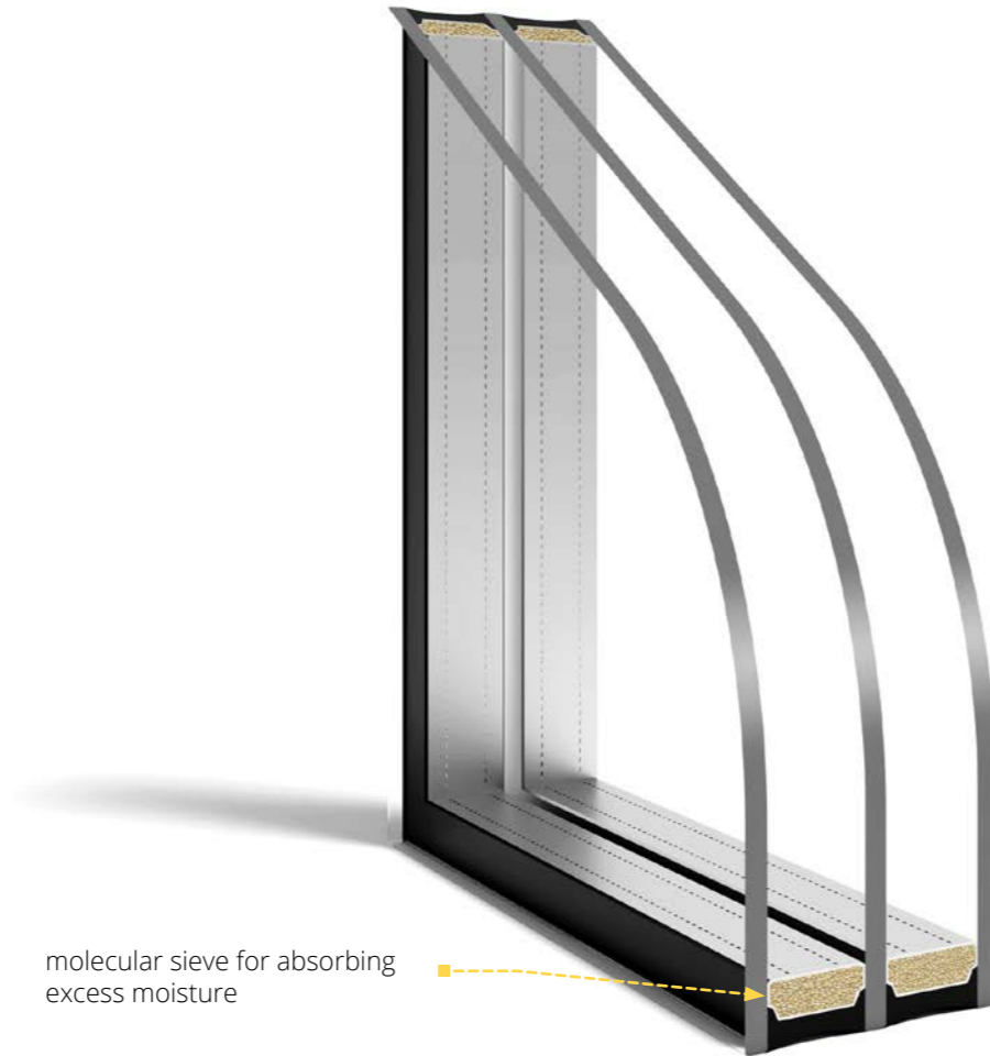
3-pane (2-chamber) 48 mm units with glass-pane spacer made of galvanised steel.
