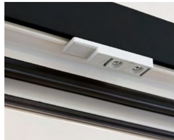
REED SWITCH magnetic window and door opening sensor is a part of the Smart Home access control system or alarm system
